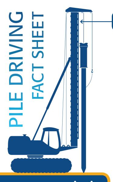
A pile driver is a device used to drive piles (poles) into soil to provide foundation support for buildings or other structures.
